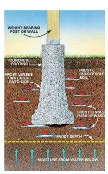
Footings that heave can create significant damage ranging from jammed doors, broken windows, cracked gypsum board, roof leaks, disconnections of plumbing or electrical work, and aesthetic implications.
