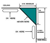
CONTAMINATE THE ALARM'S ALARM. DON'T INSTALL ALARMS WHERE AIR MOVEMENT CAN DELAY THE ALARM. THIS MEANS THEY SHOULD BE AWAY FROM WINDOWS AND AT LEAST 3 FT. FROM WARM OR COLD AIR DUCTS OR RETURN DUCTS. ALSO, DON'T INSTALL THEM BETWEEN AN AIR RETURN AND A BEDROOM DOOR.
